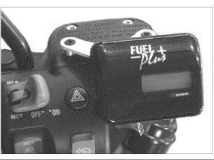
full tank or on some motorcycles it is automatic. To operate FUEL Plus ®, touch one of two invisible pads on either side of the FUEL Plus ® logo to select the functions. The touch pads will work through winter gloves and are not visible to those who might want to push buttons for fun.
