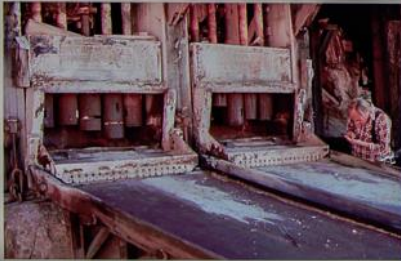
The water-powered stamps in the mill pulverized ore.
